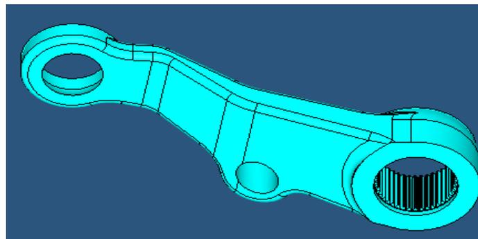
Fig. 2. Design of lift arm in .igs format as given by designer.
